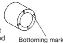
The MHSU should be used to preswage a set of ferrules only one time. If the ferrules were insufficiently preswaged, they should be discarded and the process started again with a new set of ferrules.
