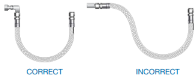
Figure 2. Avoid allowing a hose to hang vertically from a horizontal end connection. Instead, install a 90° elbow fitting.
