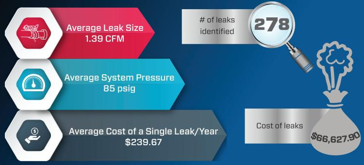
Customer's compressed gas system is online approximately 8,760 hrs/year, and the facility pays \$0.10/kWh for electricity.
