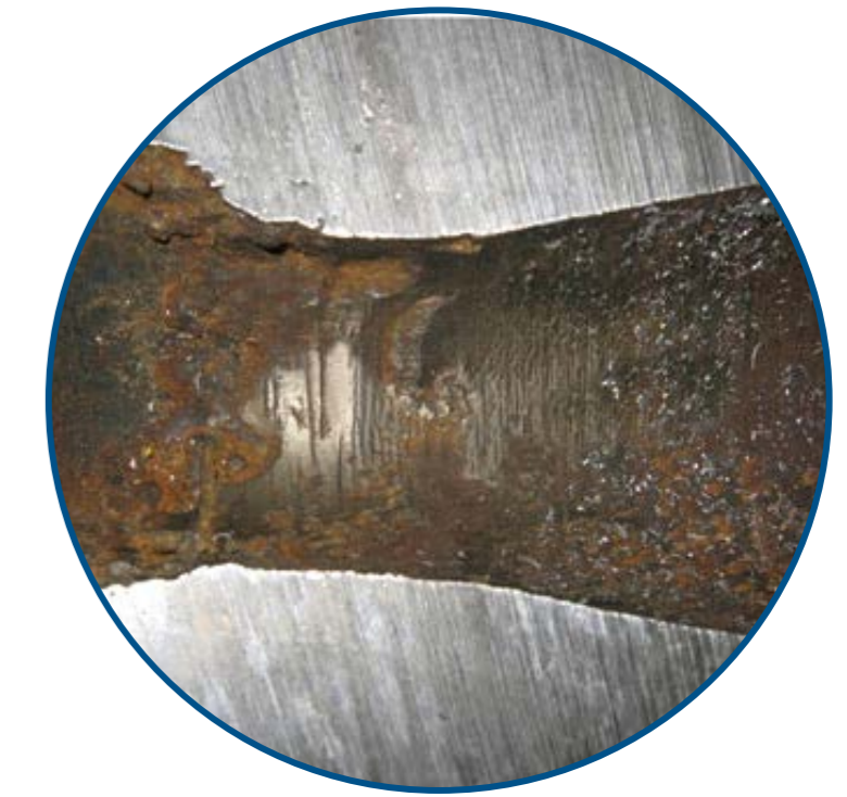
Sour Gas Cracking
