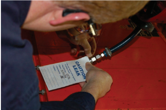
Figure 10-11 Detect and identify leaks.
