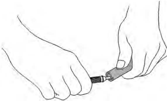
Figure 3-51 ID deburring with a Swagelok deburring tool.
