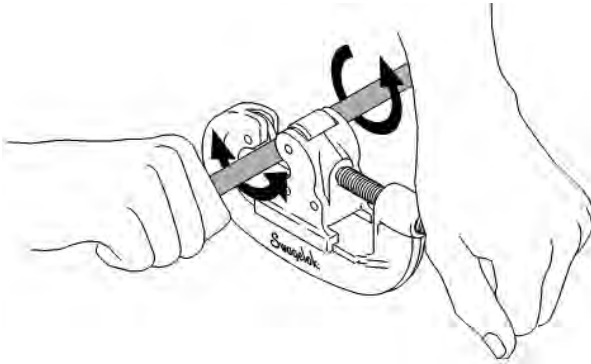
Figure 3-44 Turn the tube cutter completely around the tubing.
