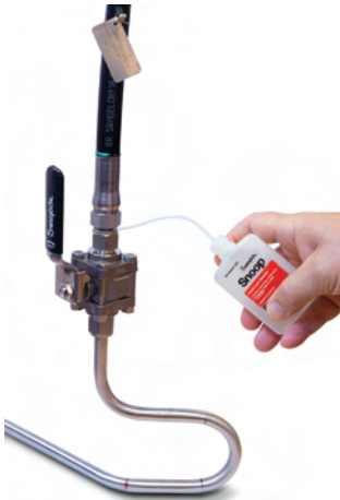
Figure 7-3 Snoop leak test.
