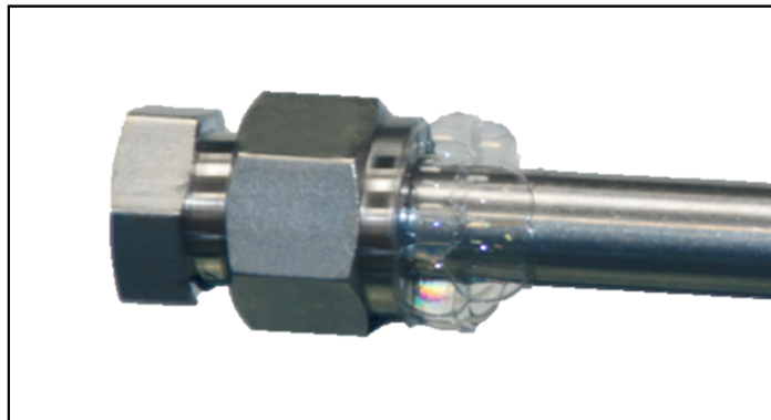
Significant loss of containment
