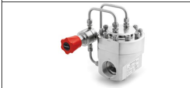
Optional: Domeloaded regulators produce flow curves with very broad horizontal sections, because they use a trapped volume of gas internally.
