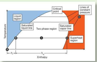
There exists a directly proportional relationship between temperature and pressure in saturated steam. That is, as the temperature increases so does the pressure. Illustrated by the "Lines of constant pressure" on the graph, more sensible energy (hf) is needed to for water to transition from point A to point B and become a vapor.
