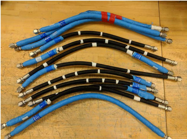
Product return at Swagelok for “pin hole” leaks at the yellow tape marks
