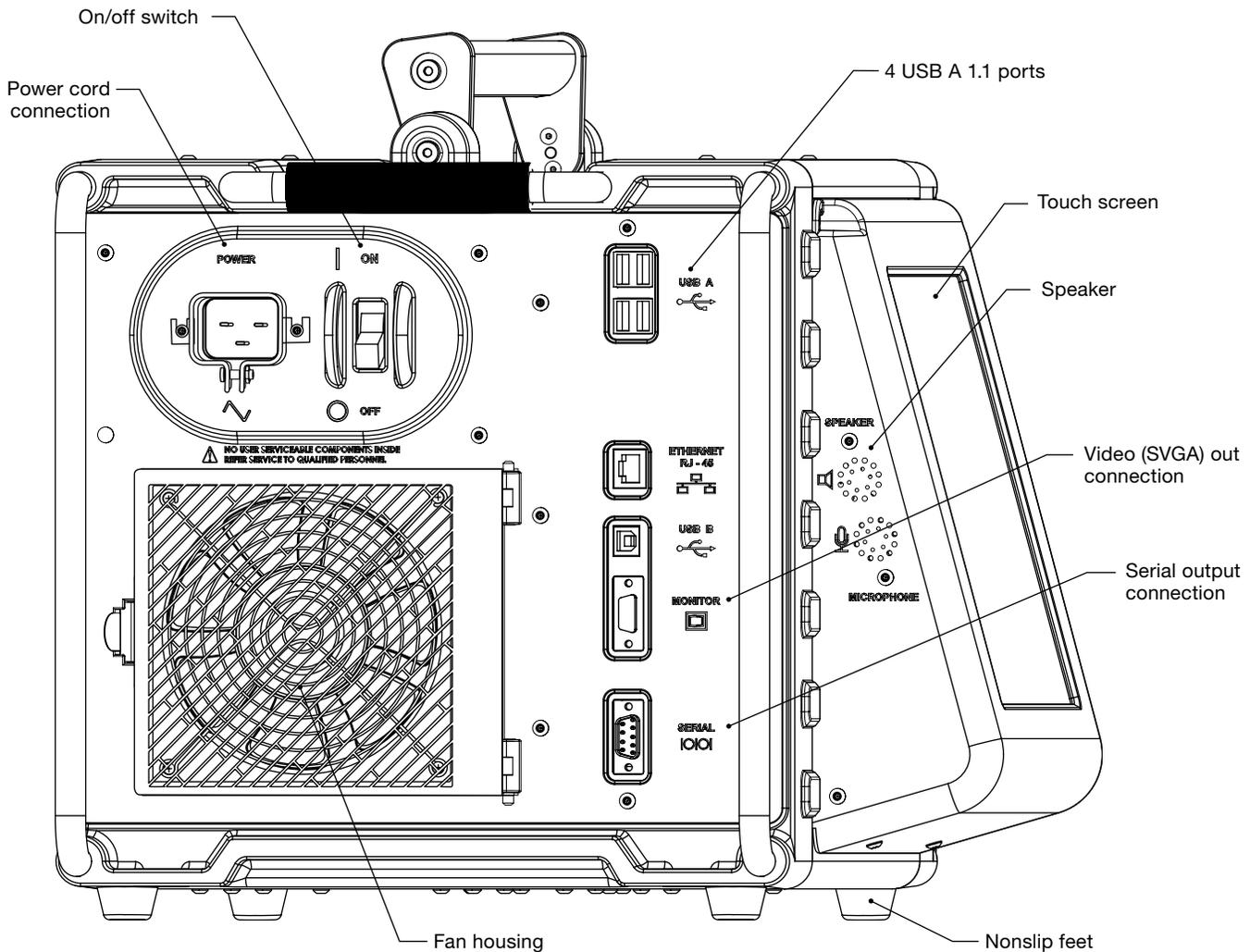
Fig. 3—M200 Power Supply Left Side
