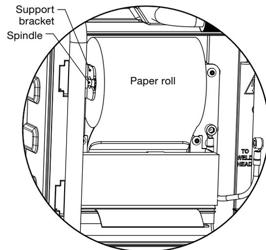
Fig. 53—Properly Loaded Paper Roll
