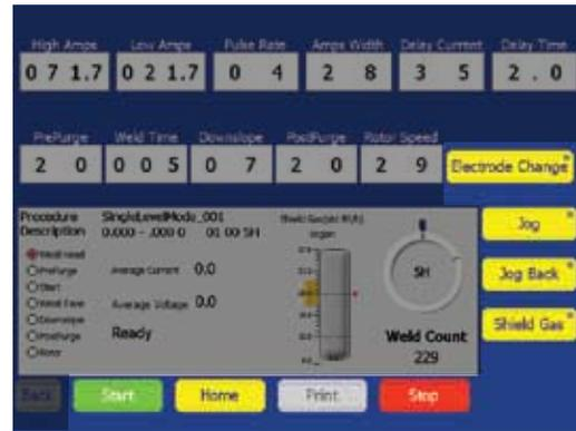
Fig. 65—Single Level Weld Process Buttons
