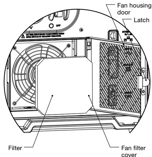
Fig. 55—Installing and Replacing the Optional Fan Filter
