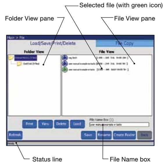
Fig. 32—Load / Save / Print / Delete Tab
