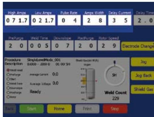
Fig. 63—Single Level Current-Control Group
