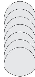
Fig. 80—Not Enough Weld-Puddle Overlap
