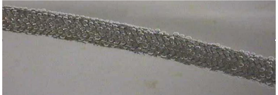
Teflon hose tested with Hydrogen in a water basin
