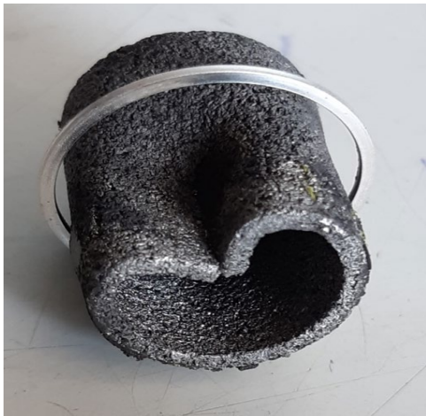
Collapsed Filter Element
