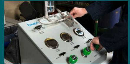
We employ a state-of-the-art Setting Station, featuring precision-calibrated gauges, to accurately set your Relief Valves at a pressure up to 1500 psi for gas service. In addition, to ensure ultimate product safety and quality, we complete a highly detailed sign-off sheet for every valve set – with a certified Swagelok inspector verifying the pressure.
