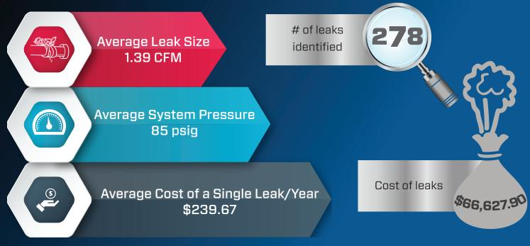
*Customer's compressed gas system is online approximately 8,760 hrs/year, and the facility pays \$0.10/kWh for electricity.*
