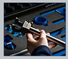
**Tee Wrench** provide positive backup support when installing Swagelok union tee and crosses, allow user to hold fitting firmly and precisely
