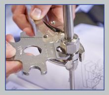
**Gap Inspection Gauge** are inserted between the nut and body of a Swagelok tube fitting after pull-up. If the gap inspection gage will fit in the gap between the nut and body hex, the fitting nut has not been sufficiently tightened.
