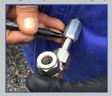
Swagelok **depth marking tools** help ensure that tubing is bottomed on the shoulder inside the Swagelok tube fitting body.
