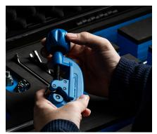
1. The Swagelok tube cutter cuts stainless steel, soft copper, and aluminum tubing from 3/16 to 1 in. and 4 to 25 mm outside diameter.
