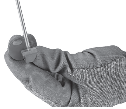
Fig. 12 Installing the Cutting Insert
