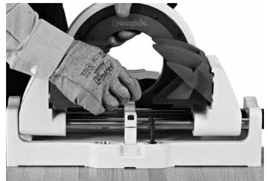
Fig 11 Attaching the Tube Cutting Tool to the Workbench
