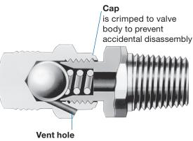
Vent hole bleeds excess liquid or gas from system lines
