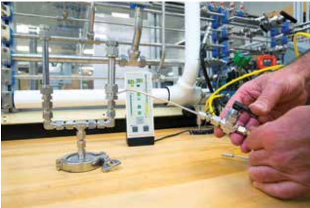
Figure 7-4 Sniffer test of helium pressurized system.
