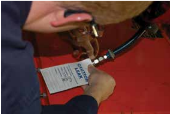
Figure 10-11 Detect and identify leaks.
