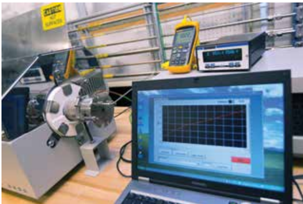
Figure 7-13 1000 psig (68 bar) gas test at 1000°F (538°C).
