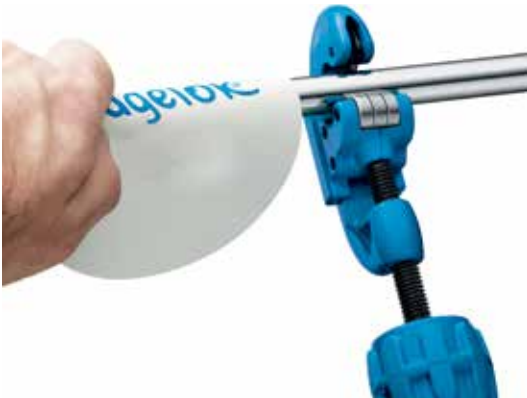
Figure 3-43 Align the cutter wheel with the measurement mark.
