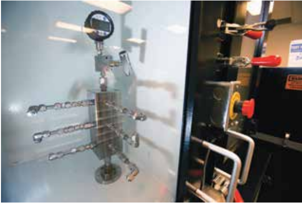
Figure 7-9 Hydraulic impulse test.
