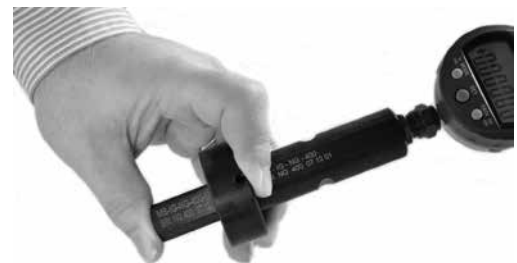
Fig. 10 Presetting the NTGS Gauge to Zero
