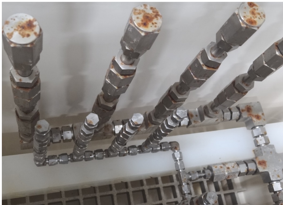
Figure 4: Pressurized FK Medium-Pressure Fittings in Cyclic Salt Spray Chamber
