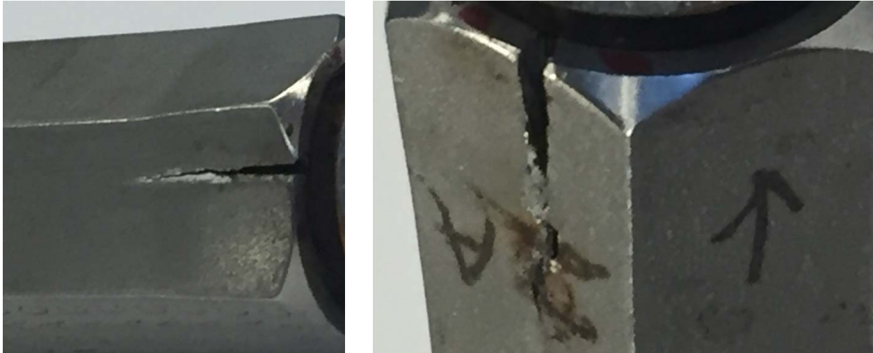
Figure 2: Examples of cracks on Another Brand's 316 SS fitting body
